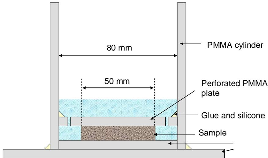
**Figure 2. Outline of the PMMA test cell.**
