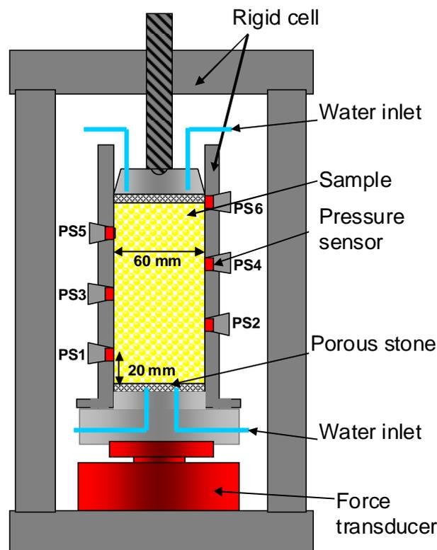
Figure 1. Layout of the mock-up test cell.
