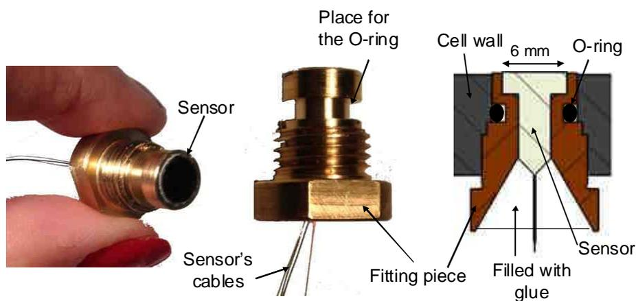
Figure 5. Total pressure sensor's fitting piece.
