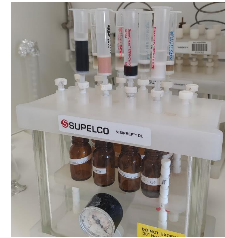
Panel of 9 commercially-available (HLB, C18, X-AW, X-CW, SDBL, ENV+, C18/ENV+, X-A, X-C) stationary phases + 1 home-made multilayer cartridge
