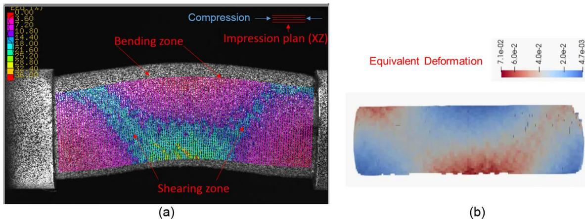
Figure 2: Equivalent strain field measured by 2D (a) and 3D image correlation (b).
