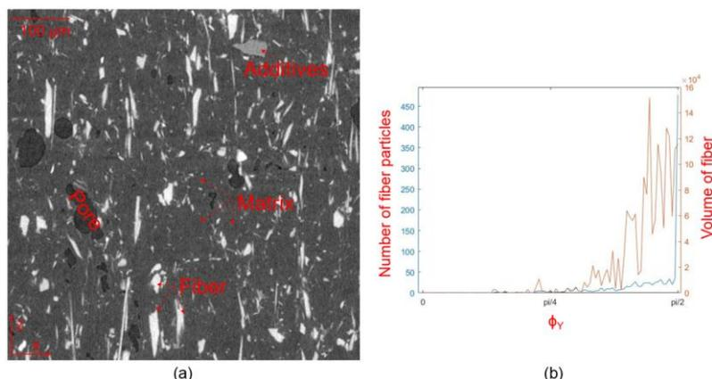
Figure 1: Cross-section along impression plane and fiber orientation distribution.
