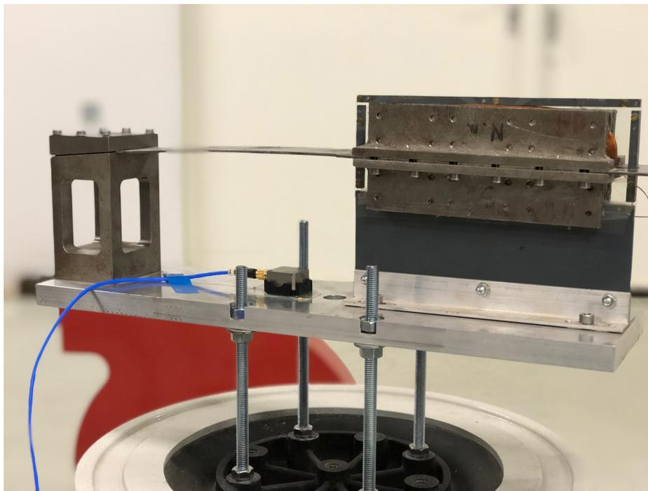
**FIG. 10.** Electromagnetic harvester.
