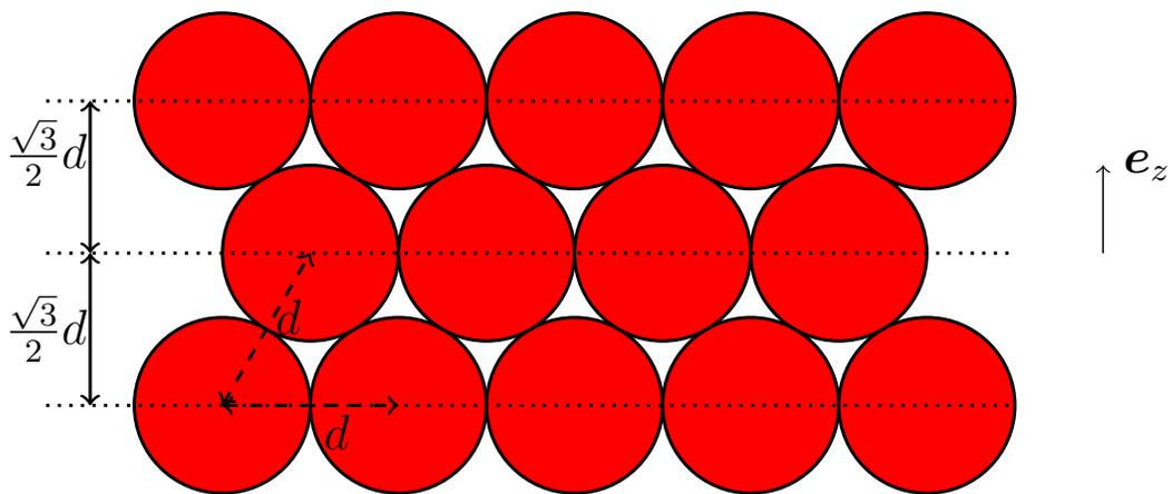
FIG. 18. Cross-section of a compact packing of wires
