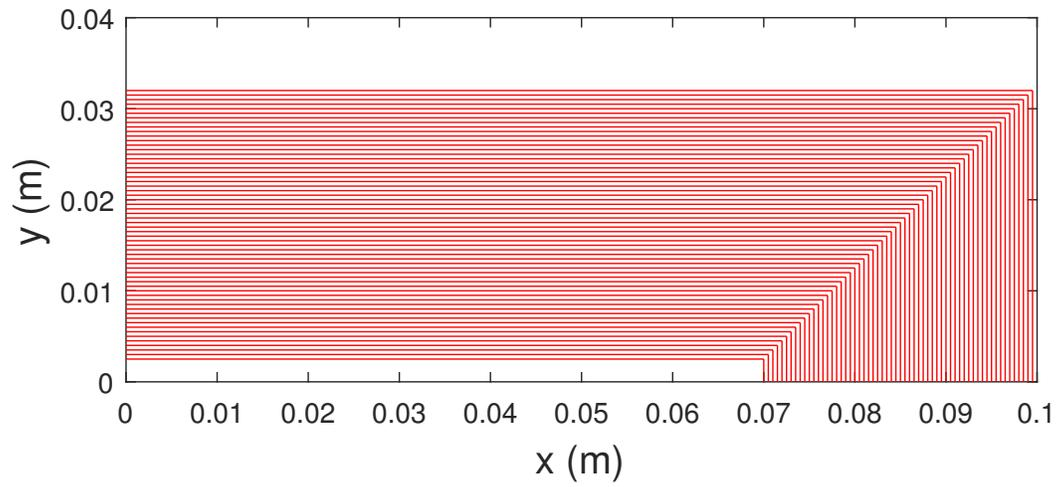
FIG. 17. Optimal coil geometry (only a quarter of the coil is shown).
