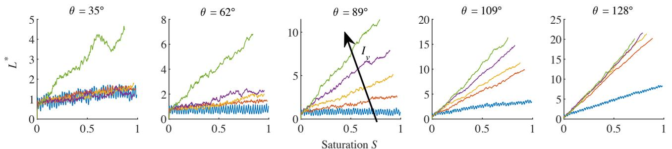
FIG. 4. Normalized fluid-fluid interfacial length ( $L^*$ ) as a function of saturation of invading fluid ( $S$ ) for different wettability and topological disorder. The black arrow indicates the direction of increasing disorder:  $I_v = 0, 0.020, 0.036, 0.047, 0.054$  corresponding to blue, orange, yellow, purple, and green curves respectively.
