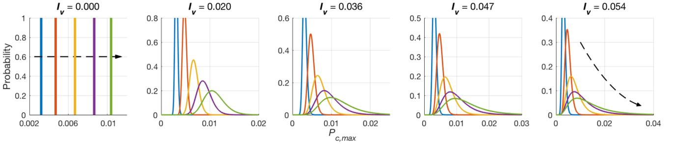
FIG. 7. Probability distribution of local maximum capillary pressure for different disorder and wettability (histogram for  $I_v = 0$  and probability density function for log-normal fitting of other values of  $I_v$ ). Black dashed arrow indicates the direction of increasing contact angle. Blue, orange, yellow, purple, and green colors correspond to  $\theta = 35^\circ, 62^\circ, 89^\circ, 109^\circ, 128^\circ$ , respectively.
