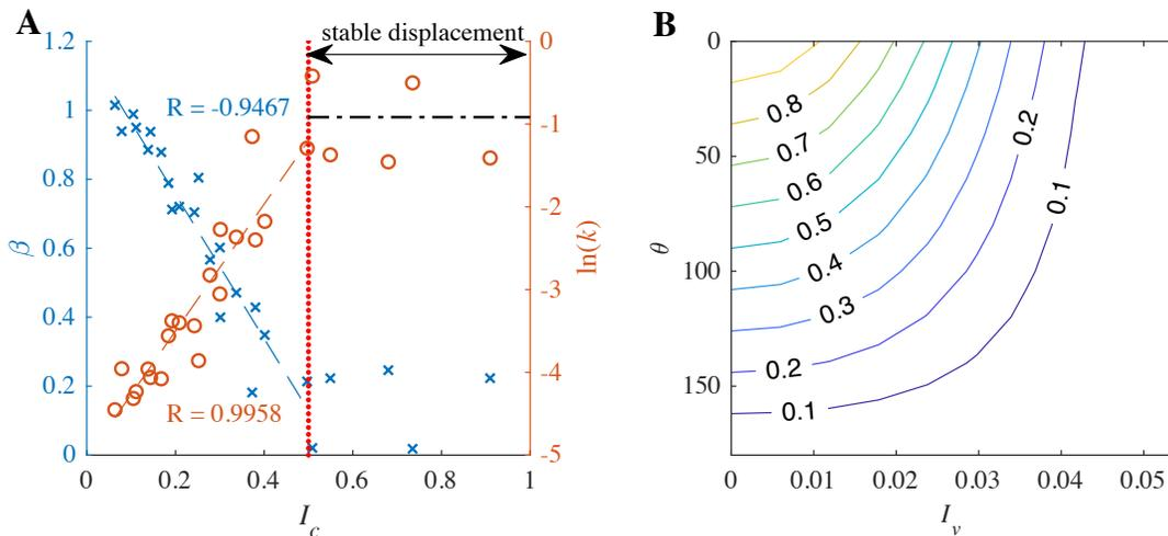
FIG. 9. (A)  $\beta$  (blue cross) and  $\ln(k)$  (orange circle) in Eqn. (9) as a function of  $I_c$ . The blue dashed line and orange solid line are the best fit lines for  $\beta$  and  $\ln(k)$  respectively. Black dashed line indicates the theoretical value for  $\ln(k)$  in perfect stable displacement. (B) Contour plot of  $I_c$  as functions of topological disorder ( $I_v$ ) and wettability ( $\theta$ ).
