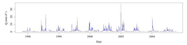
Figure 5. Hydrograph separation of the Vair River in Soulosse-sous-Saint-Élophe for 1995–2005.
