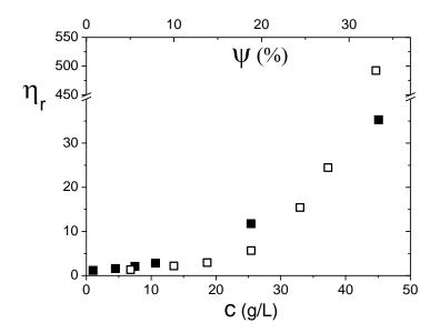
Figure 2: Relative viscosity of silica suspension in water (open squares) as a function of the volume concentration of particles (top abscissa), and of microgel suspension (filled squares) as a function of the microgel mass concentration (bottom abscissa).
