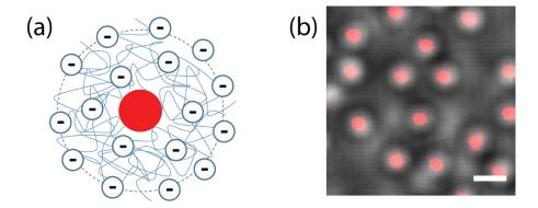
Figure 1: (a) Schematic of a microgel particle composed of a rigid fluorescent core (160 nm) and a pNIPAM structure with negative charges at pH>4.25 (pKa of acrylic acid is 4.25). Charges are throughout the structure; polymer chains extend at the surface. (b) Image of a microgel suspension (superposition of fluorescent and bright field images). The scale bar is 1  $\mu$ m.
