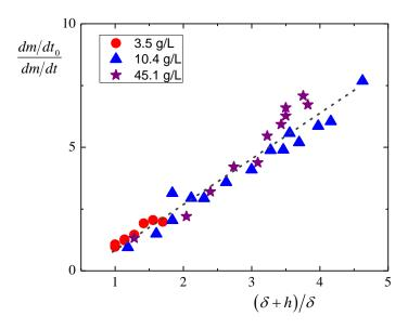
Figure 15: Bead packing filled with microgel suspensions (same symbols as in Figure 4): inverse of the drying rate normalized by the initial value as a function of the dry front thickness. The slope of the dash line is 1.5.
