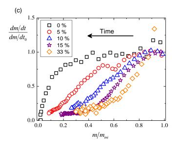
Figure 6: Drying of silica suspensions in bead packing for different concentrations: pure water (squares),  $\psi_0 = 5\%$  (red circles), 10% (blue triangles), 15% (purple stars) and 33% (orange diamonds). Water mass loss as a function of time (a) and logarithmic scale (b). Drying rate normalized by initial value as a function of **normalized water mass** (c). The colored continuous lines correspond to the migration-diffusion model (see text).
