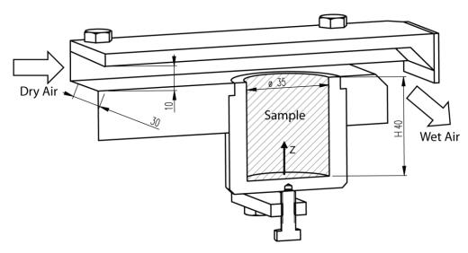
Figure 3: Design of the drying set-up in the MRI. The sample is a cylinder (H = 40 mm, diameter = 35 mm). Its upper surface is in contact with a 10 mm high channel where dry air flow at constant flux. For imaging, MRI water signal is measured along the z-axis of the sample.
