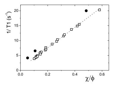
Figure 4 : NMR relaxation in silica particles suspensions. Measured 1/T1 values as a function of particle to water volume ratio (squares). Similar measurements for suspensions as interstitial fluid in a saturated bead packing (circles). The grey line is the linear fit of equation (2) for suspensions with  $\alpha = 35.2 \text{ s}^{-1}$
