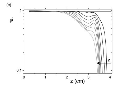
Figure 8: Drying of bead packing filled with microgel suspensions: (a)  $c_0=3.5\,$  g/L, (b)  $c_0=10.4\,$  g/L, (c)  $c_0=45.1\,$  g/L. Water saturation profiles every 10 hours after the beginning. The black line is the initial saturation.
