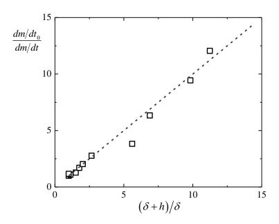
Figure 13: Bead packing filled with pure water: inverse of the drying rate normalized by the initial value as a function of the dry front thickness. The dash line is y = x.
