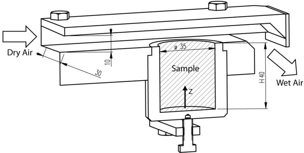
Figure 3: Design of the drying set-up in the MRI. The sample is a cylinder ( $H = 40$  mm, diameter = 35 mm). Its upper surface is in contact with a 10 mm high channel where dry air flow at constant flux. For imaging, MRI water signal is measured along the  $z$ -axis of the sample.
