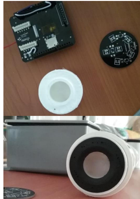
Fig. 3. Components and assembled optical sensor.
