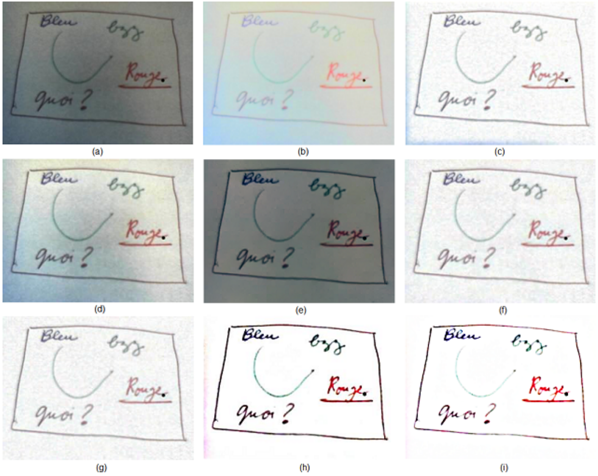
Figure 7: From top to bottom and from left to right, (a) the original image 'Board', the recovered reflectance by (b) MSRetinex [40], (c) Variational Retinex [25], (d) Screened Poisson Equation [34], (e) PDE Retinex [29], (f) local laplacian model [32], (g) the local derivatives model [32], (h) the first proposed nonlocal laplacian model, (i) the second proposed nonlocal derivatives model
