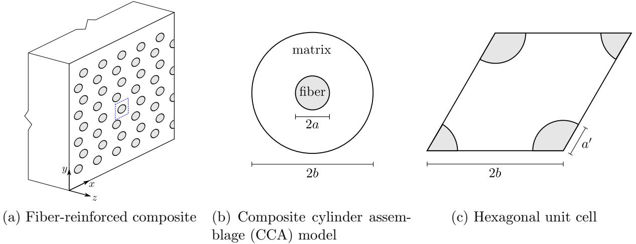
Figure 4: Unidirectional fiber-reinforced composite and associated microstructure models
