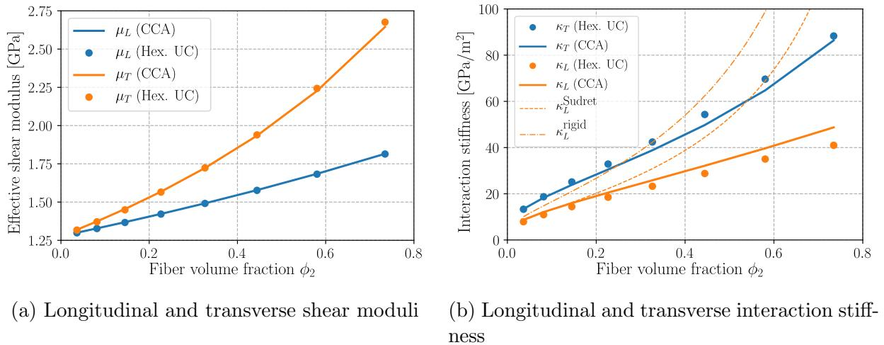
Figure 5: Comparison of the analytical predictions based on the CCA model and finite-element computations on an hexagonal periodic unit-cell for varying fiber volume fraction
