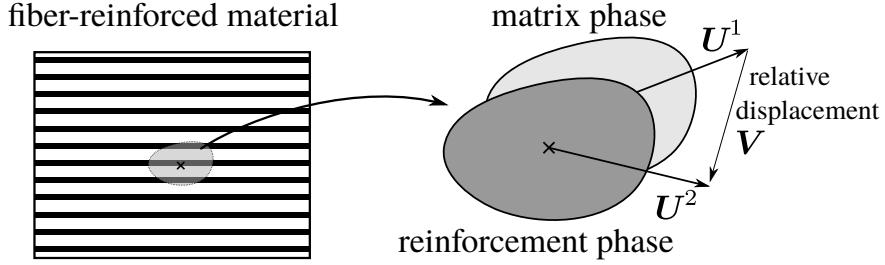
Figure 1: Fiber-reinforced material ( $N = 1$  reinforcing phase) represented by a multiphase continuum with a two-phase kinematics ( $\mathbf{U}^1, \mathbf{U}^2$ ) at any material point, interaction is described through the relative displacement  $\mathbf{V} = \mathbf{U}^2 - \mathbf{U}^1$  between both phases.
