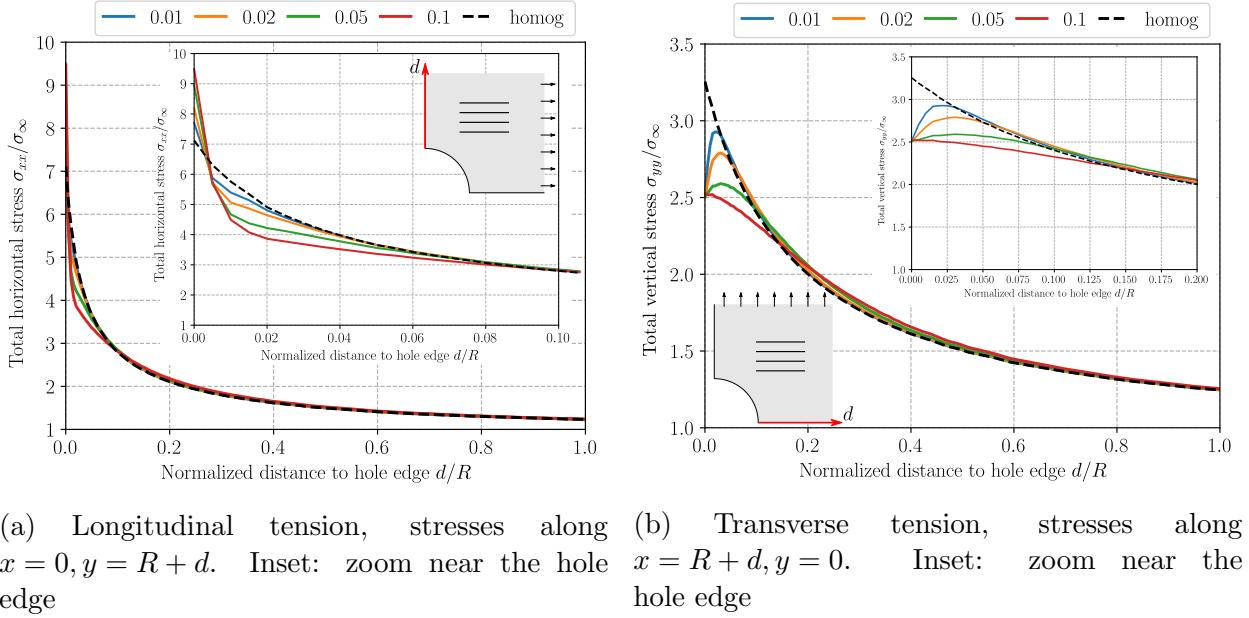
Figure 8: Total stress concentration profile near a circular hole for tension loading parallel or perpendicular to the fiber direction for varying values of the scale factor  $s/R = 0.01, 0.02, 0.05, 0.1$  and for the standard homogenized Cauchy medium (black dashed line).
