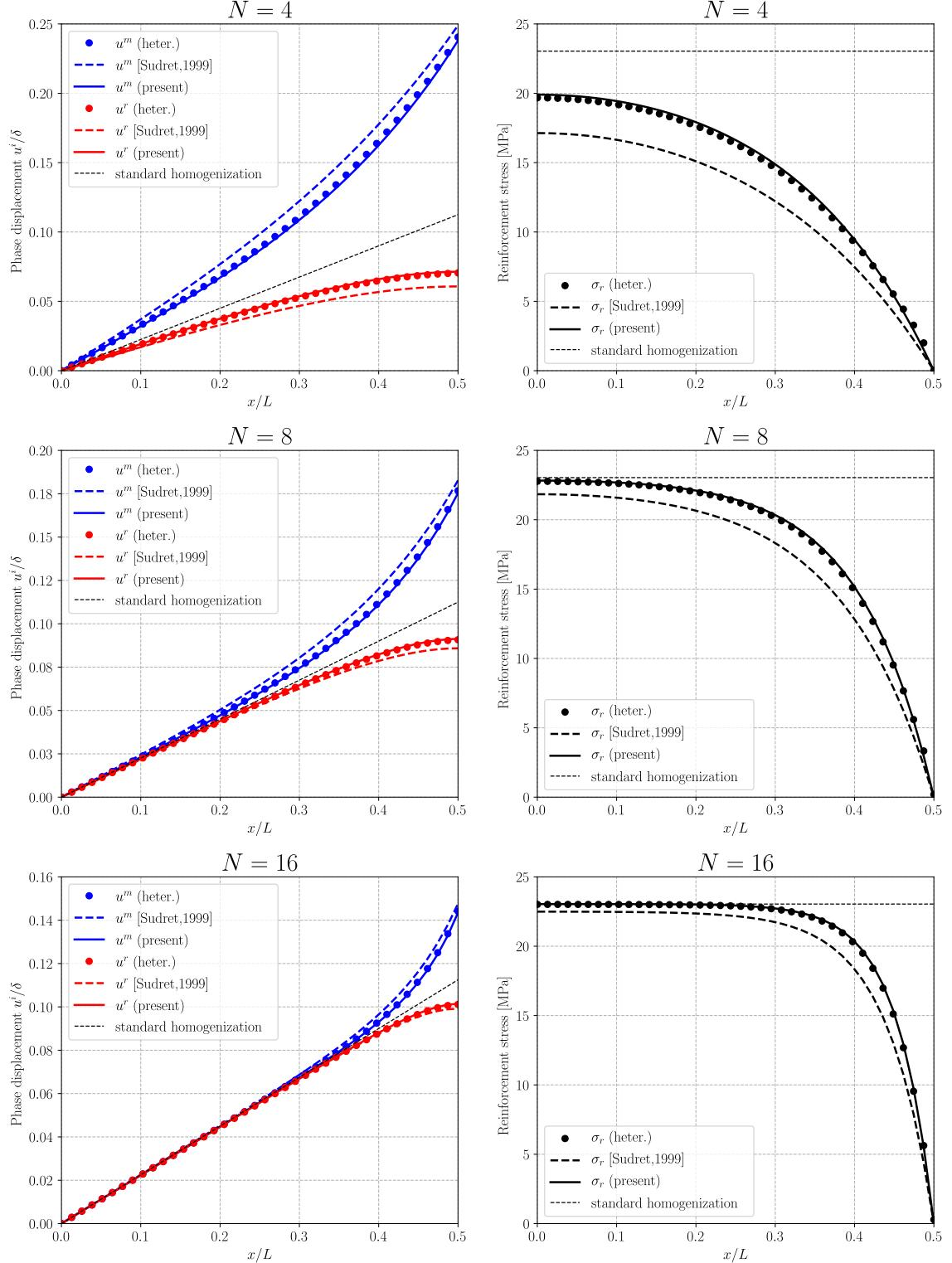
Figure 7: Comparison of matrix and reinforcement displacements (left) and partial stresses in the reinforcement (right) for different scale factors  $\epsilon = s/L = 1/N$  obtained with the original multiphase model of [52] (dashed line), the present multiphase model (solid line) and FE computations on the heterogeneous structure (symbols) with  $N$  layers.
