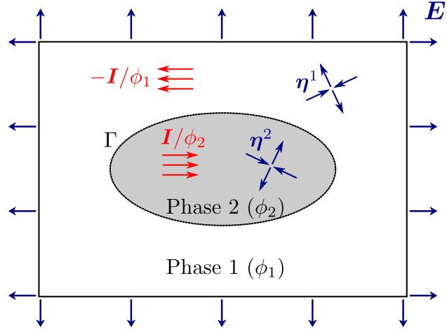
Figure 2: Auxiliary problem defined on the unit cell consisting of a macroscopic strain  $\mathbf{E}$ , self-equilibrated eigenstrains  $\boldsymbol{\eta}^i$  and body forces  $\zeta(\mathbf{y})\mathbf{I}$ .
