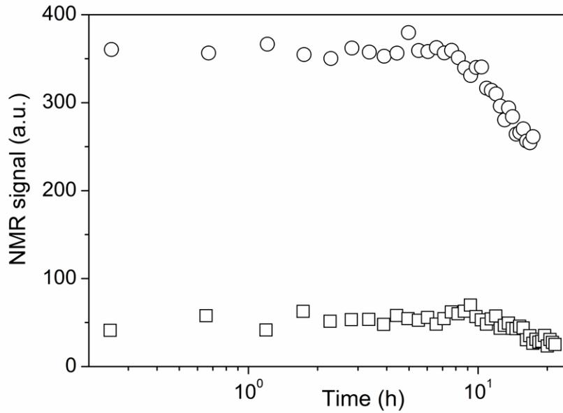
**Figure 9.** Evolution of the signal associated to water in the beads in the case of a cement paste with a W/C of 0.4 in contact with sintered beads and containing cellulose ethers (filled squares) or not (open circles) over time.
