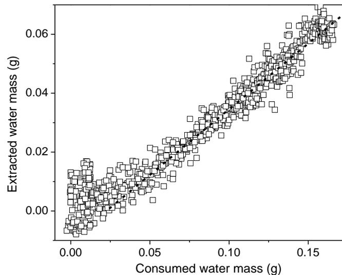
**Figure 8.** Evolution of the volume of water extracted by the cement paste from beads as a function of the consumed mass for all samples with initial W/C in the range 0.3 to 0.63. The dashed line has a slope 0.43.
