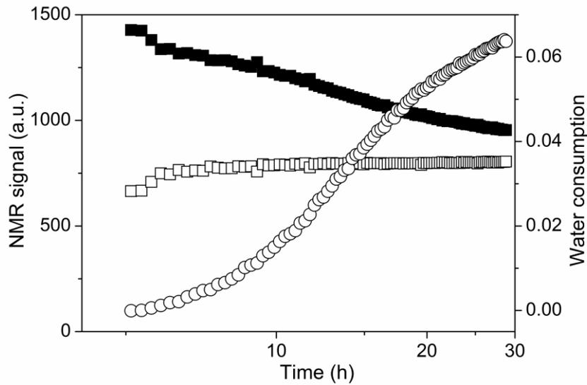
**Figure 11.** Evolution of water amount in the bead packing (empty squares) and in the paste (filled squares) as a function of time elapsed since the first contact between a cement paste (W/C = 0.5) and a silica gel. The water consumption (see text) is represented by empty circles.
