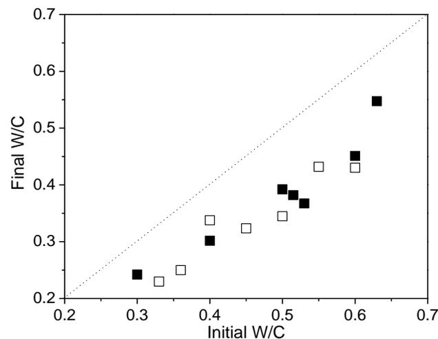
**Figure 5.** “Final” W/C (i.e. after the first period of contact between the paste and the bead packing) as a function of the initial W/C for the cement paste. Empty squares for packing A, filled squares for packing B.
