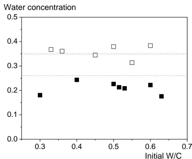
**Figure 4.** Water volume fraction in the bead packing (empty squares for packing A, filled squares for packing B) after the initial period of contact with a cement paste as a function of the initial water to cement ratio of the paste. The dotted lines correspond to the porosity of each bead packing.
