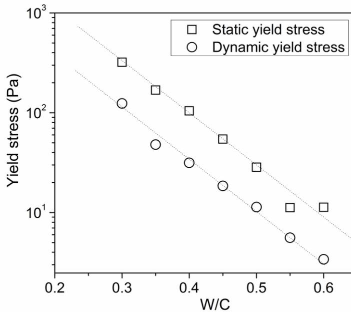
**Figure 1.** Evolution of static and dynamic yield stresses of a cement paste as a function of the water to cement ratio. The dotted lines correspond to negative exponential functions fitted to data (see text) fitted to each set of data. For the largest W/C value (i.e. 0.63) reliable rheometrical data could not be obtained.
