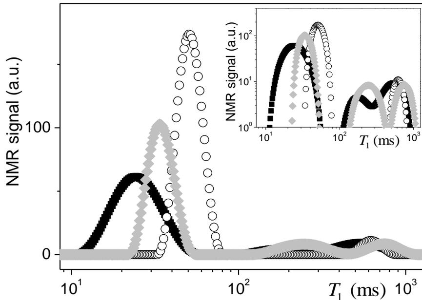
**Figure 3.** Distributions of relaxation times for a paste in contact with a bead packing (A for cement, B for the two other materials) for cement paste (W/C=0.5) (diamond), kaolin paste (squares) and bentonite paste (circles), during the first 30 min. The inset shows the same data in logarithmic scale.
