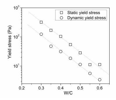
**Figure 1.** Evolution of static and dynamic yield stresses of a cement paste as a function of the water to cement ratio. The dotted lines correspond to negative exponential functions fitted to data (see text) fitted to each set of data. For the largest W/C value (i.e. 0.63) reliable rheometrical data could not be obtained.
