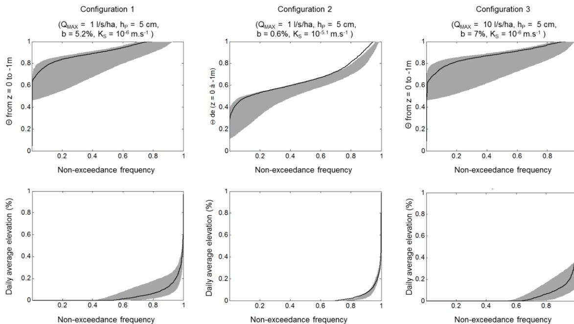
Figure 5 – Distribution of the average relative water content  $\Theta$  in the first 100-cm of soil (average values over 24h) and distribution of the daily average water elevation (expressed as percentage of the maximum water elevation) (10-90% confidence intervals)
