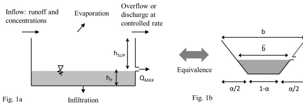
Figure 1 – 1a. Representation of the source control system 1b. Effect of the cross-sectional shape parameter  $\alpha$  (the introduction of  $\bar{b}$  is justified later on)
