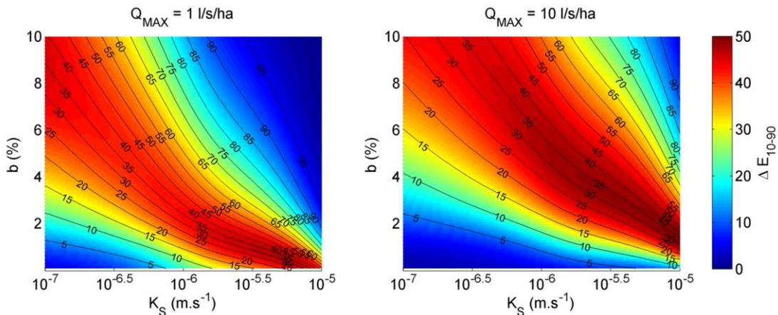
Figure 2 – Sizing diagrams for  $h_P = 0$  and  $Q_{MAX} = 1$  and 10 l/s/ha (contour lines = 10<sup>th</sup> percentile of simulated efficiencies,  $\Delta E_{10-90}$  = difference between the 90<sup>th</sup> and the 10<sup>th</sup> percentile of simulate efficiencies)
