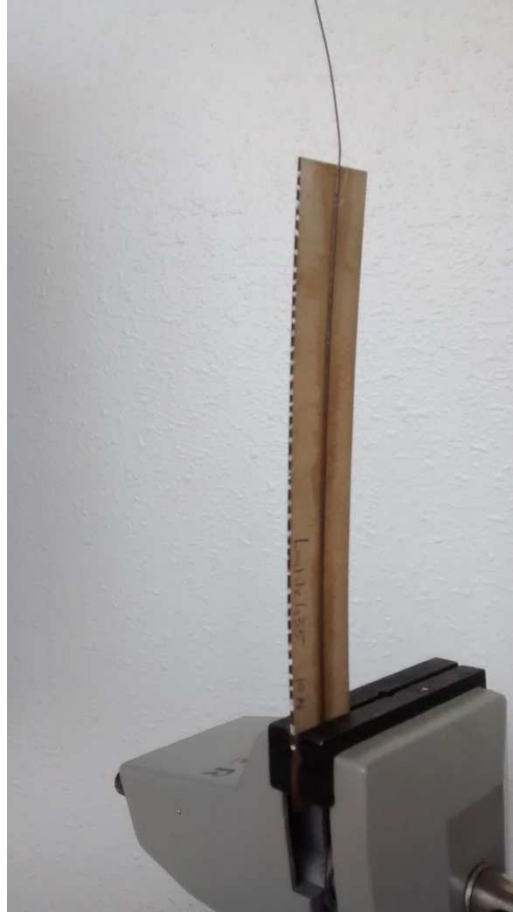
Fig. 1. Bilayer-type actuator composed of a wooden lamella and an SMA wire: initial state at ambient temperature
