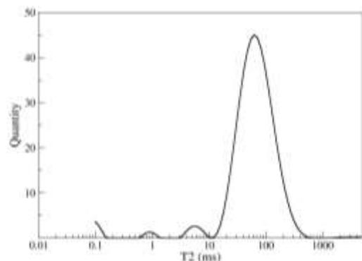
Fig. 3. Distribution of the T2 relaxation time inferred from NMR on the Lavoux limestone.
