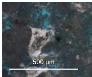
Fig. 1. Thin section of Lavoux limestone in white light microscopy. (a) Oolite (b) Pellet (c) Syntaxial cements (d) Bioclast. The porosity appears in blue due to colored epoxy saturation.
