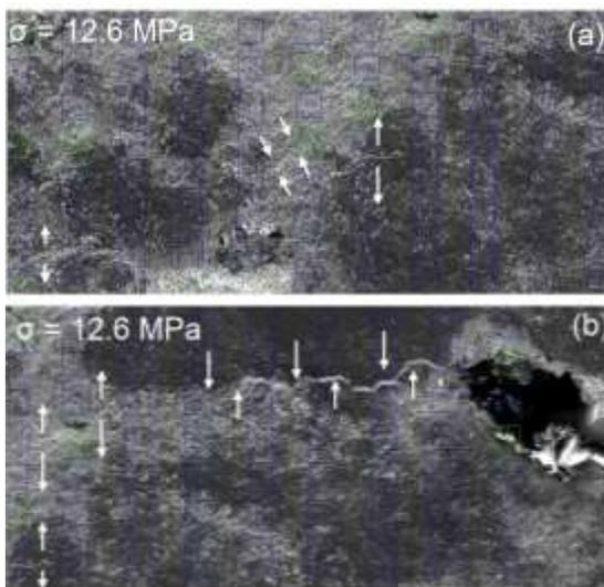
Fig. 14. (a) Extensive and compressive cracks and (b) Extensive cracks developed at grain interface in area reported on Fig. 7. (b) Whites arrow directions highlight the opening or closure of cracks.
