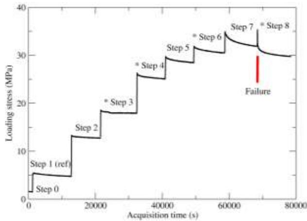
Fig. 18. Loading curve of the test performed on the intact sample at a confining pressure of 5 MPa. The steps pointed out by a star correspond to ones reported in Fig. 20
