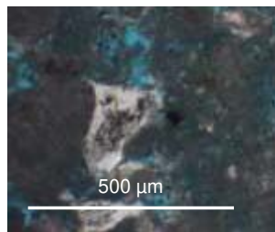
Fig. 1. Thin section of Lavoux limestone in white light microscopy. (a) Oolite (b) Pellet (c) Syntaxial cements (d) Bioclast. The porosity appears in blue due to colored epoxy saturation.
