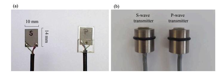
Figure 3. Bender elements transducers: (a) wiring of two bender elements; (b) GDS bender elements waterproofed and encapsulated in pot
