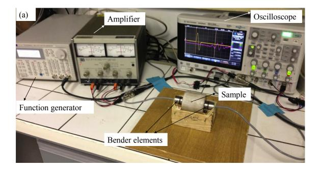
Figure 4. Setup of the bender element testing: (a) photo of the setup; (b) schematic diagram of the setup
