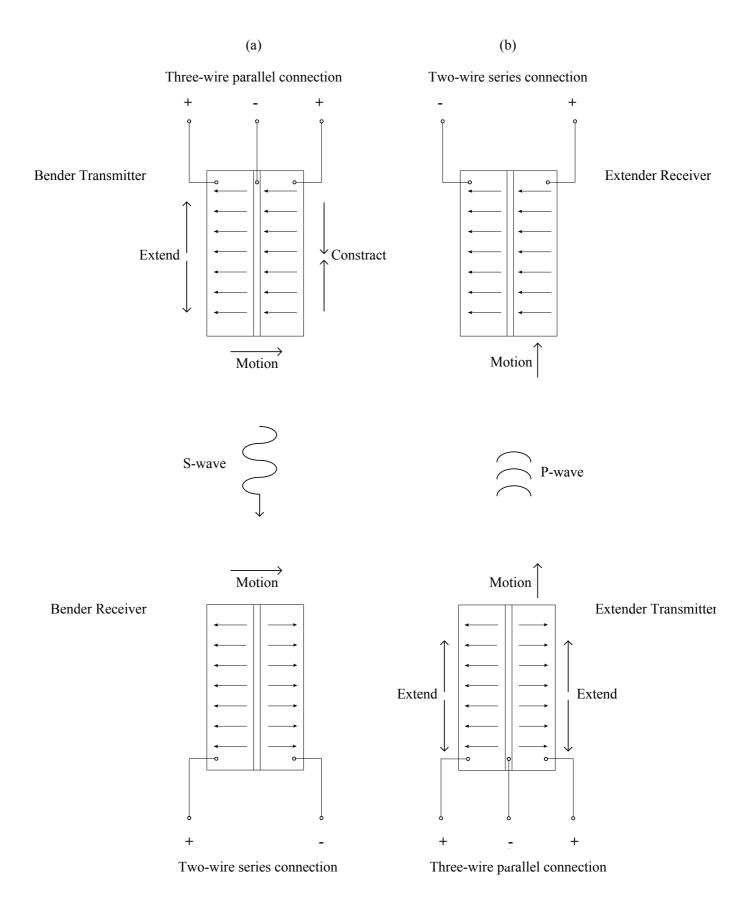
Figure 1. Sketch of bender and extender connection: (a) transmitting S-wave; (b) transmitting P-wave (after Lings and Greening 2001)
