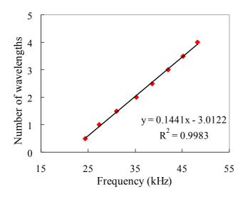
Figure 6. Measurements by "π-point" method on a lime-treated soil (D1)
