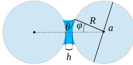
**FIG. 1.** A meniscus between two spherical grains of diameter  $a = 2R$ , with distance  $h$  between solid surfaces, filling angle  $\varphi$ , contact angle  $\theta$ .
