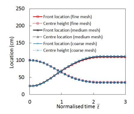
Figure 14. Effects of the utilized mesh size on the curves for front location and centre height
