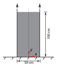
Figure 10. Schematic diagram for the collapse of a column of sensitive clays
