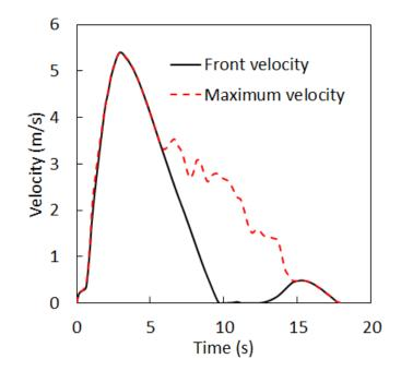
Figure 18. Velocity of the sliding front and the maximum velocity against time
