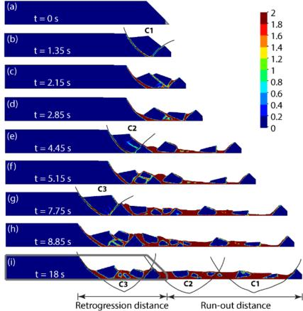
Figure 17. Retrogressive failure procedures of the slope. Colours are proportional to
