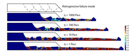
Figure 20. Final deposits from the simulation using different viscosity coefficients for
