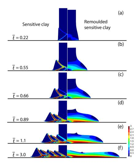
Figure 11. Collapse evolution processes of the column of initially undisturbed sensitive clays
