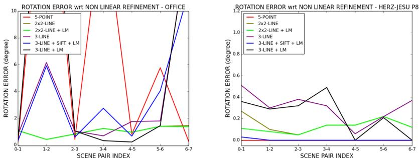
**Fig. 6.** Rotation error for image pairs in datasets *Office* (left) and Strecha’s *Herz-Jesu-P8* (right). Reported methods do not use their final refinement stage (Levenberg-Marquardt, LM) unless otherwise mentioned. The curve for “ $2 \times 2$ -lines + LM” is often hidden by the “ $2 \times 2$ -line” curve.
