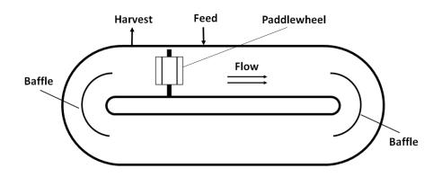
Figure 2. Plan view of a raceway pond
