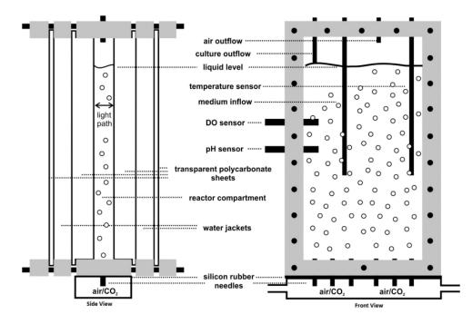
Figure 5. Front and side views of flat photobioreactor (Bahadar and Bilal Khan, 2013)
