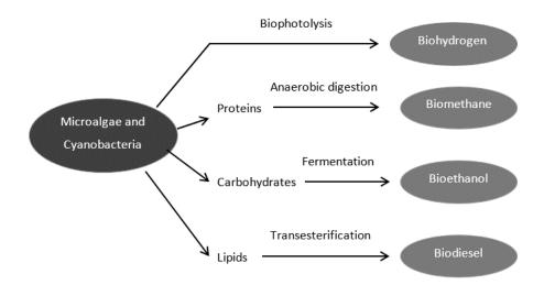
Figure 7. Types of biofuel produced from microalgae and corresponding technologies
