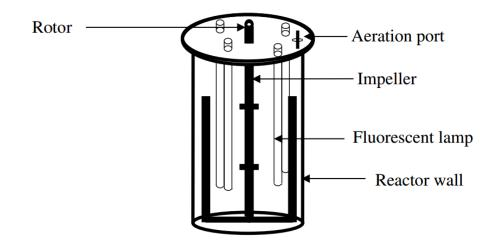
Figure 6. Internally-illuminated photobioreactor (Ugwu et al., 2008)
