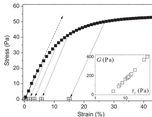
FIG. 2. Creep test for an emulsion ( $\tau_c = 54$  Pa): (filled squares) stress vs strain when applying a stress ramp; (crossed squares) final strain after stress release (no stress imposed) at some point during the ramp; dotted lines, stress-strain path. Inset:  $G$  measured in the region of negligible final strain after stress release, as a function of yield stress, for emulsions at different concentrations; the dotted line corresponds to  $G = 140 \ln(\tau_c/3.2)$ .
