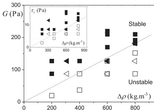
FIG. 3. RTI results for YSF in terms of elastic modulus as a function of density difference for  $L = 7$  cm (triangles) or  $L = 15$  cm (squares): stable cases (filled symbols), unstable cases (open symbols). The dotted line is a guide for the eyes. The inset shows the same data represented in terms of  $\tau_c$  with the corresponding dotted line (consistent with the  $G$  vs  $\tau_c$  variation) and a straight dashed line as a guide for the eye.
