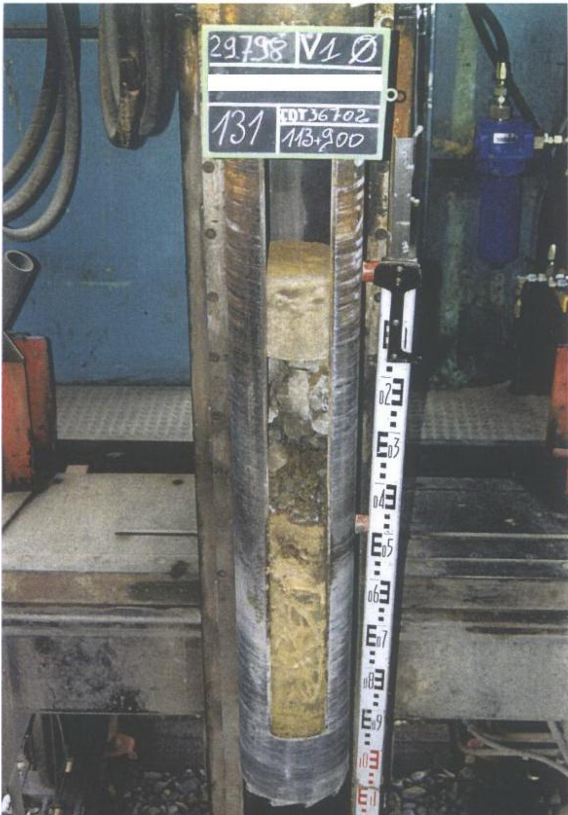
Fig. 10: Core sample from typical conventional railway sub-structure
