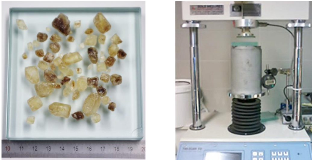
Figure 5. Left: Rock sugar grains (particles) of various sizes. Right: Single-grain crush test apparatus.
