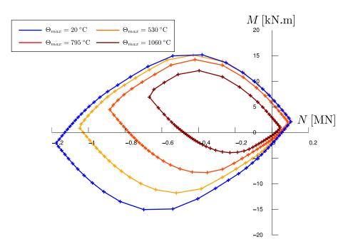
Figure 9: Evolution of the  $N_{11} - M_{11}$  interaction diagram with respect to the temperature
