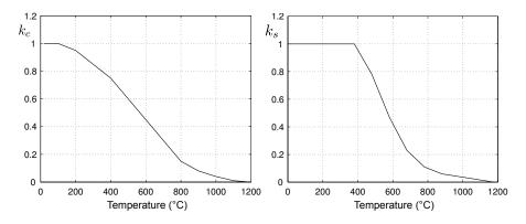
Figure 6: Reduction factors for concrete (left) and steel (right) as a function of temperature
