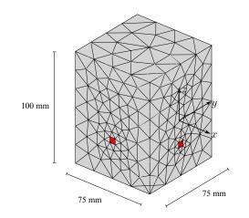
Figure 7: Unit cell geometry and mesh for the second example
