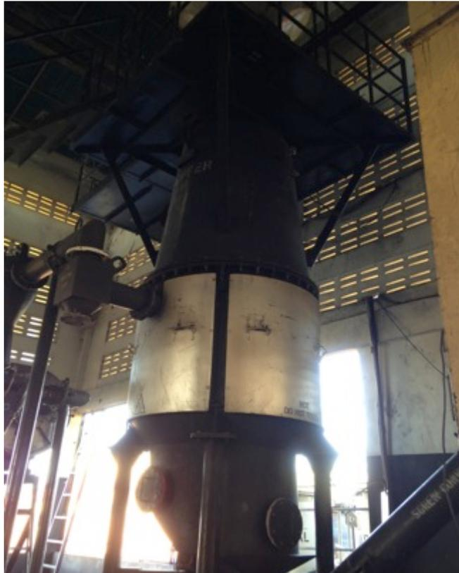
**Figure 8:** 150kW Ankur downdraft gasifier at UNIDO Project, Siem Siep Province, Cambodia, 2014-12-20
