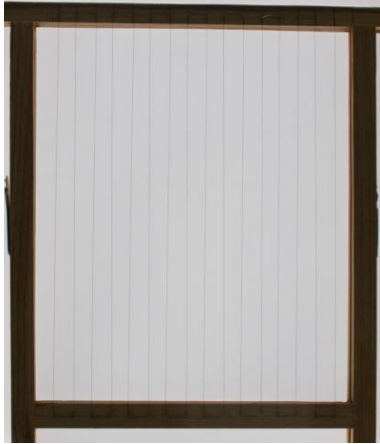
Figure 1. Calibration harp of Tang [12], used to compute the distortion field.
