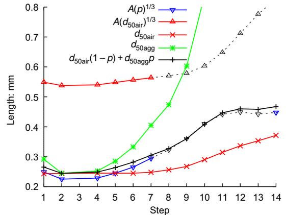
**Fig. 7.** Median diameter of air and aggregate phases as a function of wetting step. The figure shows the cube root of the air fraction integral range (blue triangles when  $b > 0.9$  and grey dashed lines when  $b < 0.9$ ), the cube root of the integral range of the air median diameter (red triangles) and the sum of the median diameters weighted by the fraction of their complement (black lines with  $p$  the air fraction)
