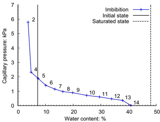
**Fig. 1.** Capillary pressure at top of specimen as a function of macroscopic water content. The initial state (black solid line) at 7.2% water content and the ‘theoretical’ saturated state (black dashed line) at 48% are plotted. Each blue cross corresponds to an equilibrium state at which a scan of the specimen was acquired
