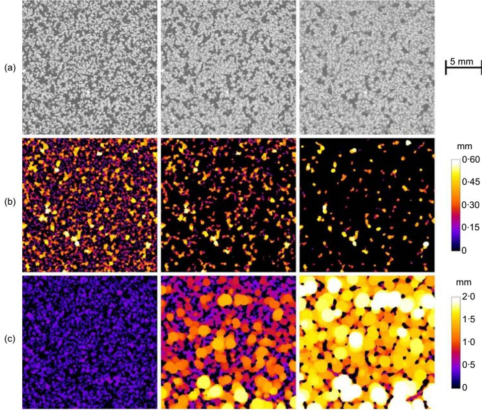
**Fig. 3.** Maps of a vertical slice of the isolated volume after reconstruction (a), after thresholding and application of Matheron's granulometry on the air phase (b) and on the aggregate phase (c). Colour scales give the value of the diameter of the biggest 3D inscribed spheres (in mm)
