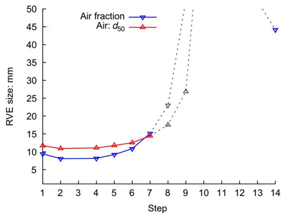
**Fig. 8.** RVE size of air fraction and of median diameter of air as a function of the considered step. RVE size is the side length of the cube giving a relative expanded uncertainty of 1%. Grey lines correspond to the steps at which the isolated volume was heterogeneous
