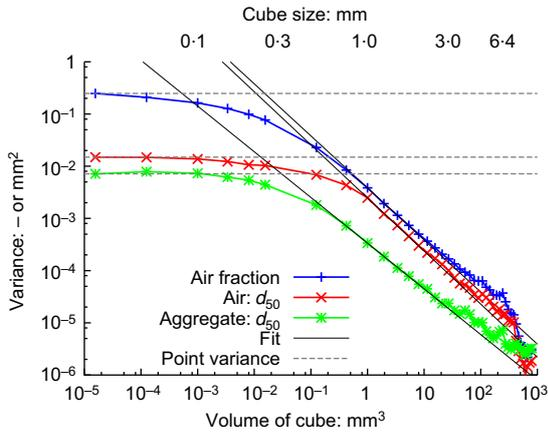
**Fig. 4.** Variance (dimensionless) of air fraction and variance (in  $\text{mm}^2$ ) of median diameters at the initial state. The dashed lines plot the point variances and solid lines the fits of the variances using equation (1)
