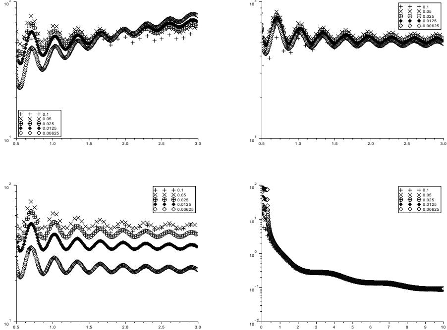
Figure 1: For  $\Delta t = .1, .05, .025, .0125, .00625$ , effectivities in log scale (as a function of  $T$ ) of (20) – top left –, (22) – top right –, and (23) – bottom left – ( $\|\operatorname{div} \mathbf{u}^{\Delta t}\|_{L^\infty(0,T;Q)}^2$  included) at estimating (19) when  $\lambda = 10, T \leq 3$ ; and  $\|\operatorname{div} \mathbf{u}^{\Delta t}\|_{L^\infty(0,T;Q)}^2 / \text{error } (19)$  – bottom right – when  $\lambda = 1, T \leq 10$ .
