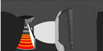
**Figure 9:** Stairway detection on simulated LiDAR data.
