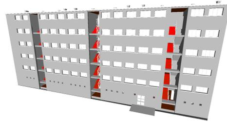
**Figure 3:** Automatic stairs detection in LcC building.
