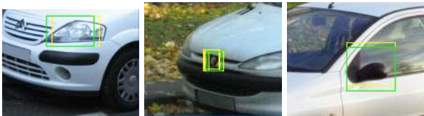
Figure 5: Examples of detections. Last column is a false detection, as a rear mirror of the wrong model is detected. This kind of false detection is expected to happen repeatedly and is a reason for the noise on the signature.
