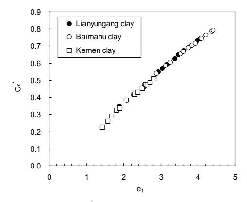
Fig. 5. Relationship between  $C_c^*$  and  $e_I$  for three reconstituted clays at different initial water contents
