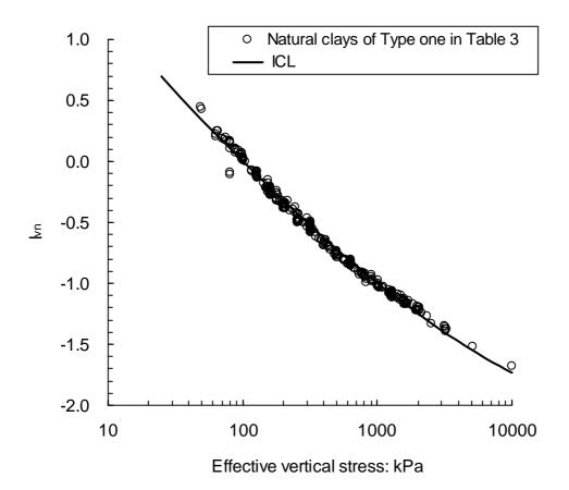
Fig. 18. Normalised behaviour with void index  $I_{\nu n}$  for natural clays of Type one in post-yield regime
