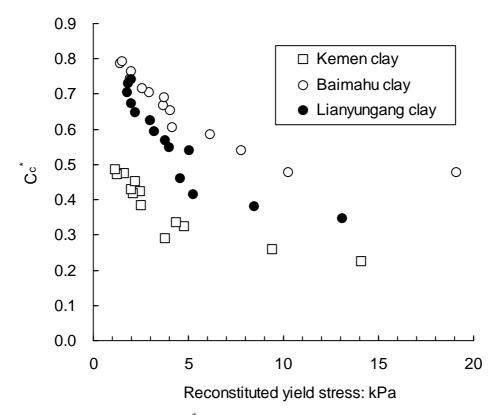
Fig. 3. Relationship between  $C_c^*$  and  $\sigma_{yr}$  for three reconstituted clays at different initial water contents
