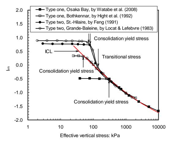
Fig. 17. Typical normalised behaviour with void index  $I_{vn}$  for two types of natural clays listed in Table 3  $\,$
