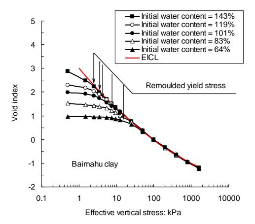
Fig. 8. Typical  $I_{\nu} - \log \sigma_{\nu}'$  curves of reconstituted clays at different initial water contents
