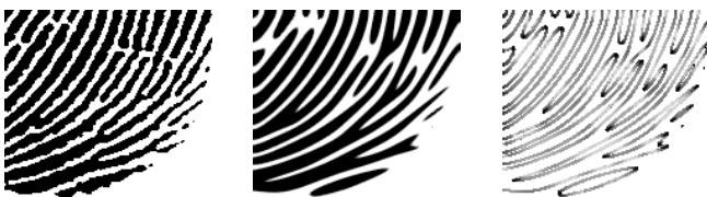
(a). Fingerprint (b). LLS evolution (c). Curvatures
