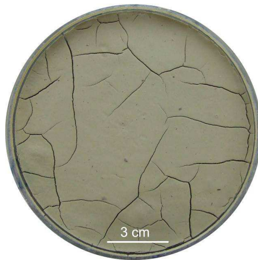
29 Fig. 2 A typical desiccation crack pattern of specimen during the first
