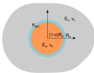
Fig. 1: Aggregate and surrounding cement paste
