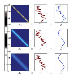
FIG 1. The effect of the smoothing matrix  $A_{\lambda}$  on the resulting estimator. In this example, the true signal is the sine function over  $[-\pi,\pi]$  and the three matrices represented in the leftmost column are some powers of one convolution matrix. Large powers correspond to stronger smoothing. One clearly see that the third matrix leads to an almost perfect recovery of the original signal.
