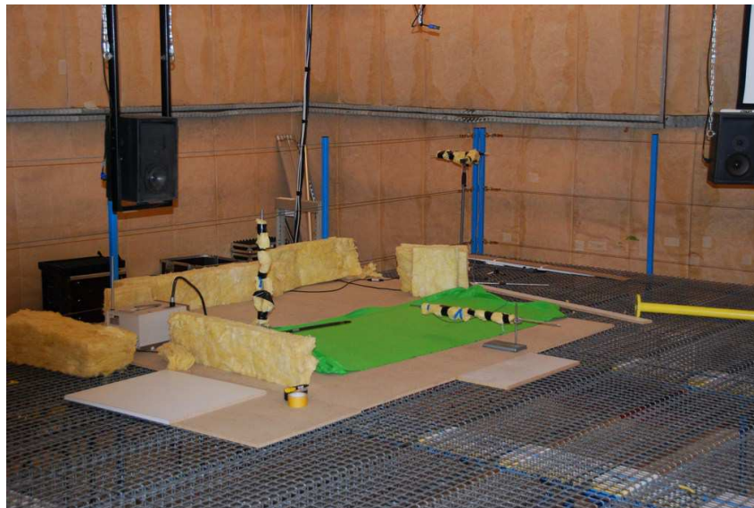
Figure 7.4: Overview of the experimental set up in the “scale model room” at the CSTB Grenoble. The walls of the room are covered with absorptive glass wool, which makes the room rather dry. Besides, the noise floor is low thanks to good insulation.
