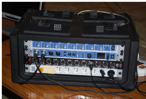
Figure 7.9: Fireface UFX soundboard used to acquire the signals from the receiver microphone and the reference microphone. Maximum sampling frequency is f_s = 192 kHz.
