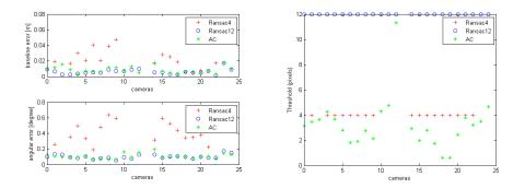
Fig. 4. Evaluation of camera pose estimation with RANSAC and AC-RANSAC on HerzJesusP25. Two views are first registered with a fundamental matrix, yielding a 3D point cloud. Then the pose of all other images is computed relatively to that point cloud. Thresholds 4 (Bundler's default) and 12 are tested. On the left is displayed the pose error relative to ground truth (baseline, angle), on the right the used thresholds.
