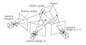
Fig. 2. Structure from Motion.
